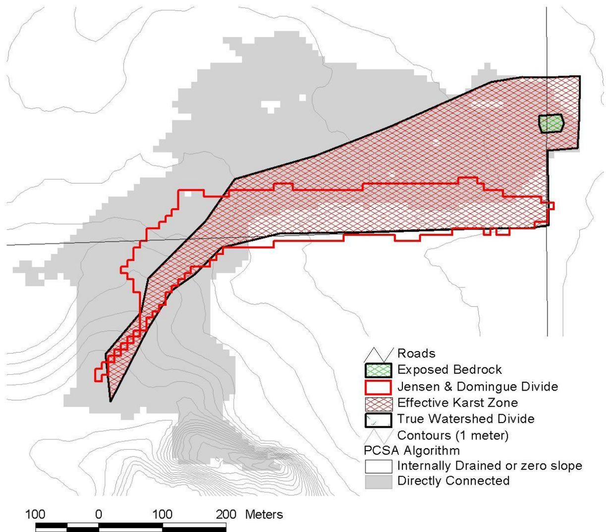
**Figure 31** Site 62; an exposed fracture-bedrock zone. 100% of its watershed is covered with thin soils.
