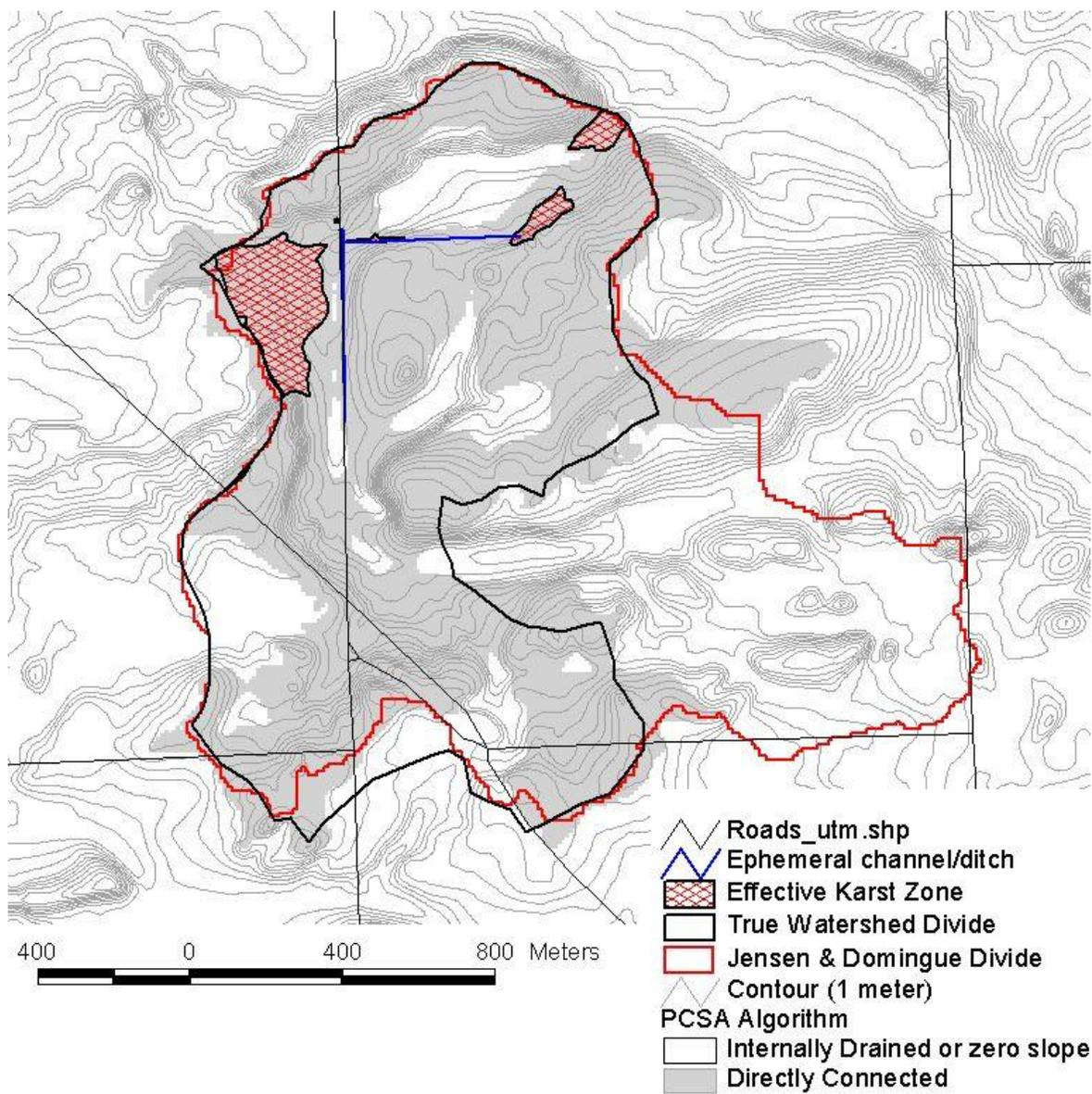
**Figure 11** Site 15a; a solution sinkhole. Drainage in this feature is augmented by a drainage ditch along Townline Rd.
