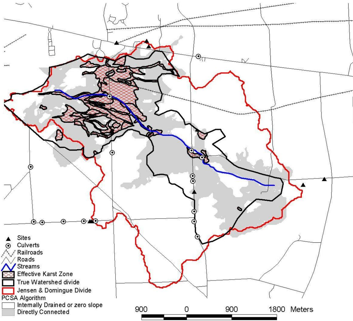
**Figure 10** Site 15; a complex thinly soiled karst system composed of multiple thinly-soiled karst features. Site of the 2007 well contamination event.
