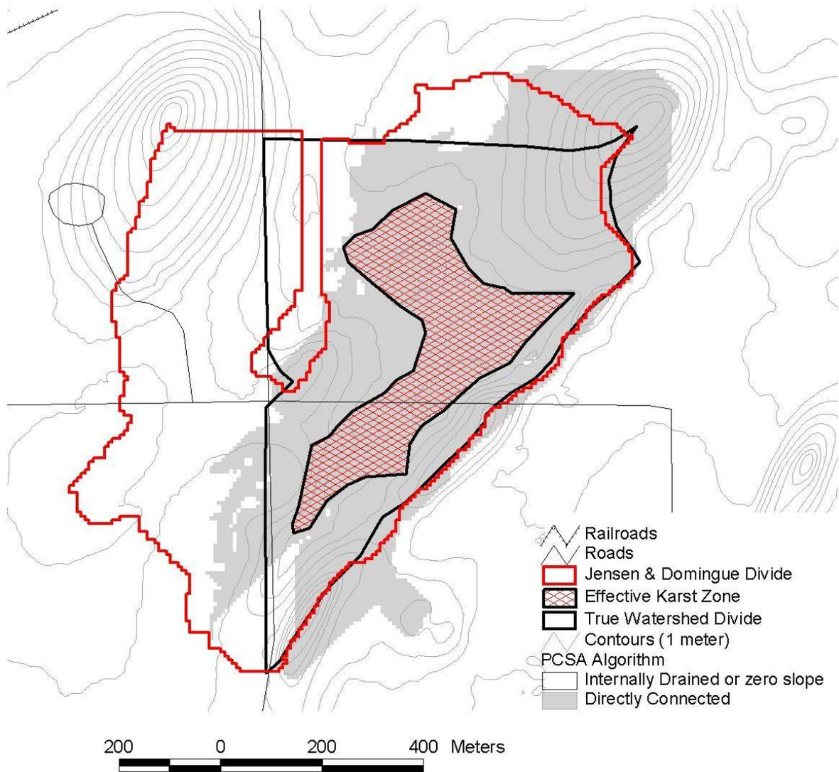
**Figure 6** Site 9; originally classified as a glacially enhanced sinkhole, this sinkhole has been reclassified as a glacial feature because of the absence of bedrock and thick overburden in the site.
