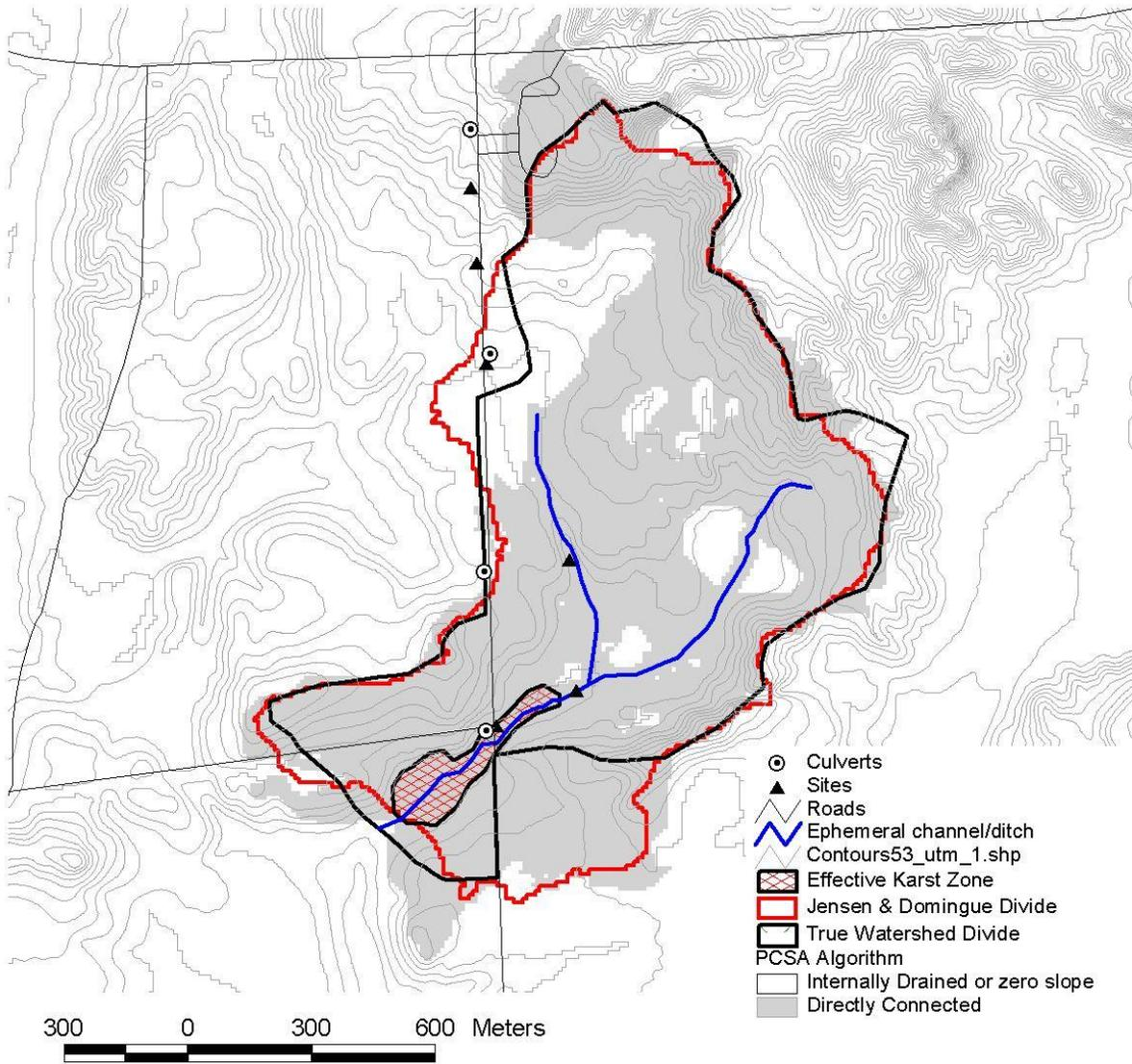
**Figure 26** Site 53; a glacially enhanced sinkhole system.
