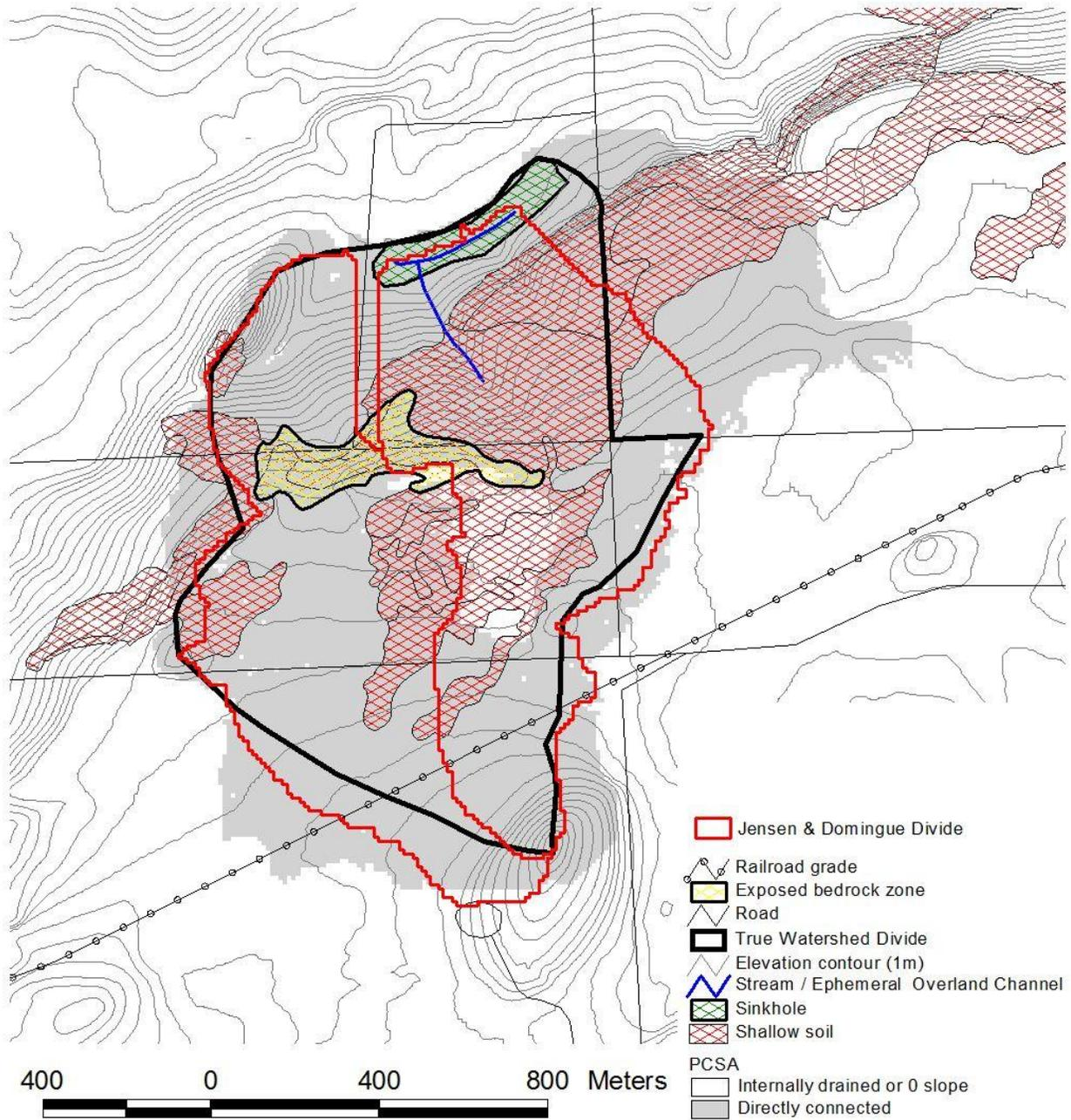
**Figure 8** Site 11; the Buckley Rd. sinkhole system. Contains fractured bedrock and a solution sinkhole located on a fracture trace.
