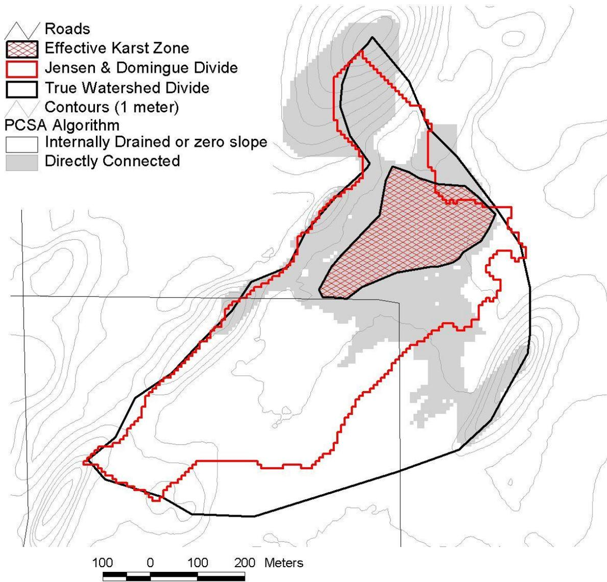
**Figure 7** Site 10; originally classified as a glacially enhanced sinkhole, this sinkhole has been reclassified as a glacial feature because of the absence of bedrock and thick overburden in the site.
