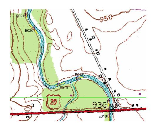
Erosion here is mostly occurring near the bridge. Sediment has collected at erosion points E016 and E017, forcing water to the opposite side of the collected sediment.
