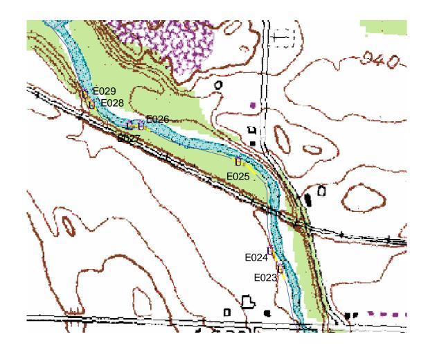
In this section there are no erosion points of immediate concern. Most erosion is a result of deposition along the banks which forces water towards the other bank. At erosion points E030 and E031, erosion is occurring on the left bank. The right bank of E032 is undergoing erosion.
